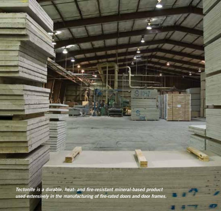
*Tectonite is a durable, heat- and fire-resistant mineral-based product used extensively in the manufacturing of fire-rated doors and door frames.*
